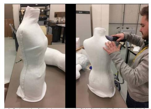
Left: Fosshape tube after placing on mannequin. Right: Steaming the fosshape to make it form to the mannequin.
